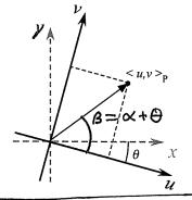
\* Note well: V-axis has been rotated toward point P, as compared to Y-axis
