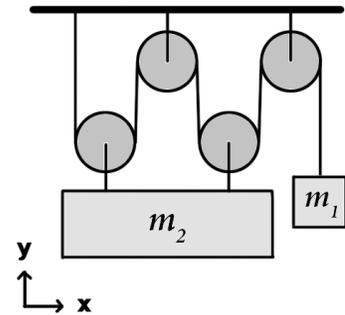
If object  $m_1$  moves a distance  $d$  in a particular time, the object  $m_2$  can only move one-fourth as far. Each of the four segments of rope supporting  $m_2$  will change their length by  $d/4$ . That is sufficient to choose
